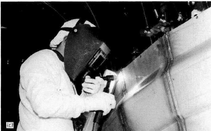
15 Semi-automatic TIG welding: a) Equipment for automatic feeding of the filler wire; b) Vacuum vessel of the Joint European Torus (JET) ; c) Manual TIG welding of the stainless steel inner lining of the toroid vessel (b and c courtesy of the JET Joint Undertaking).
